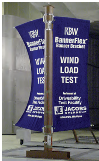
BannerFlex Wind Tunnel Test
